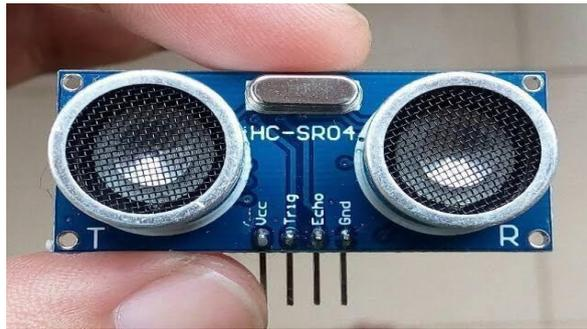
Gambar 4. Sensor ultrasonik
