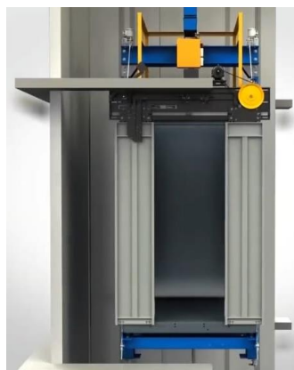
Gambar 2 Desain pintu center opening
