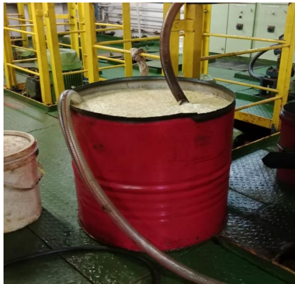
Gambar: 5. Chemical Flushing system FWM Sumber: FC. Winning Sunrise
