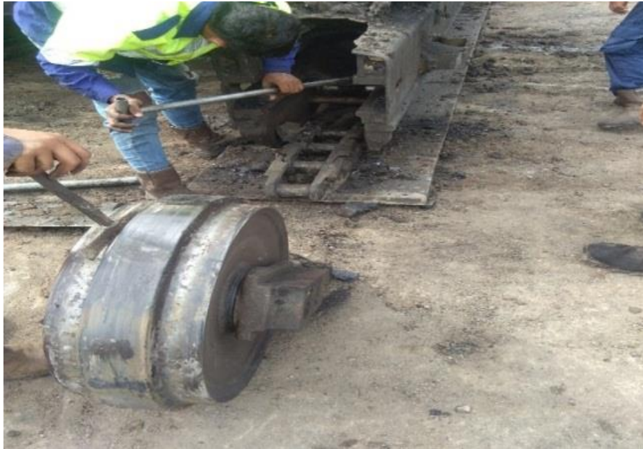
Gambar 4.3: Pergantian recoil spring
