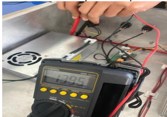
Gambar 12 Pengukuran Output DC Power Supply
