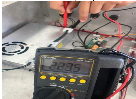
Gambar 11 Pengukuran Input Power Supply
